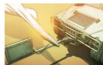
4 / BOMB-PROOF ADJUSTMENTS (FALL 2006) The Rhino II, which costs less than \$2,000 and has an adjustable-length boom, changes the position of the decoy. More than 16,000 Rhino IIs are deployed overseas in just 30 months.
