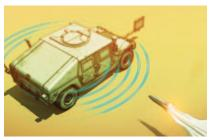
JAMMER-TRIGGERED BOMBS (EARLY 2010) New EFPs ignore heat signatures and are triggered by the high-power radio waves emitted by coalition jammers. In other words, the latest bomb is set off by the countermeasure that defeated its predecessors.
